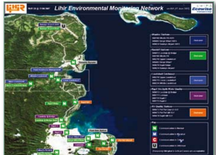
After collection by LoggerNet the data is displayed using web pages generated by RTMC Web Server. These are available to all LGL staff via a link on the Lihir intranet.
