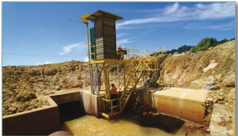
Water Quality stations around the pit provide information crucial to the safe and efficient operation of the mine.
